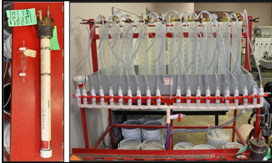
Figure 6.45: PVC core sample gas desorption canister and slow desorption testing apparatus
