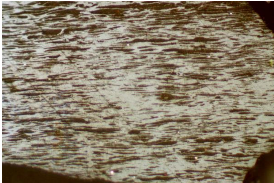
Figure 4.9 Tahmoor coal with abundant clay filled cell lumen in vitrinite. Reflected white light image; Field width = 0.54 mm
